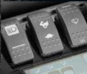
*The speed-selection switch is now located on the right-hand console, providing more room for tired feet. The switch eliminates the need to hold down a pedal during high-speed transport.*
