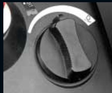
*A new rotary dial throttle is equipped with an auto-idle function. Release controls and in four seconds the engine rpm drops to idle, saving fuel and reducing noise. Touch a control, and engine rpm returns to the preset level.*
