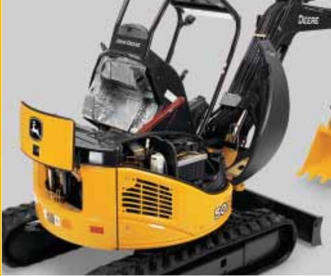
The operating station tilts forward 50 degrees, reducing service time by providing easy access to the control valve and front-side engine components.
