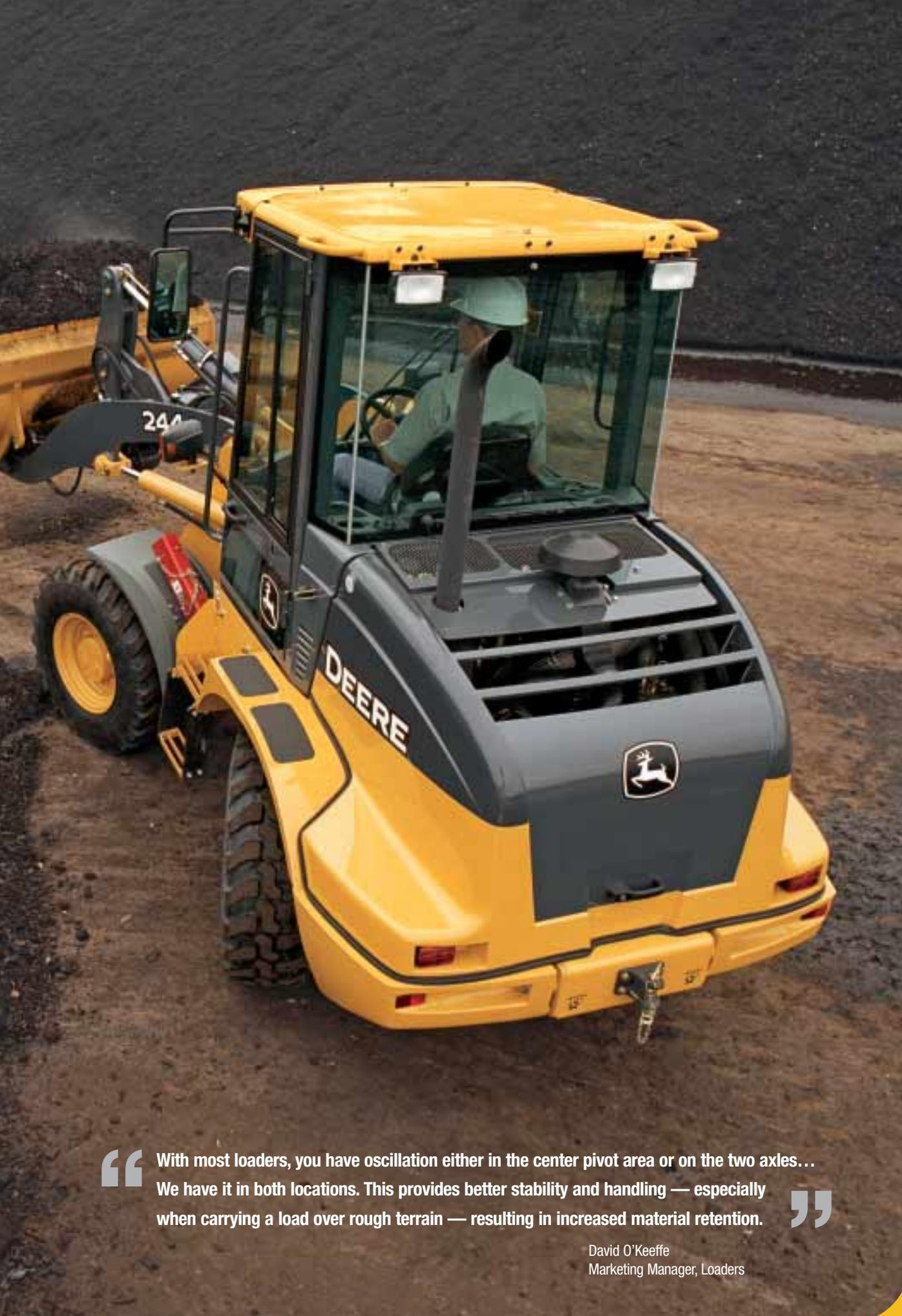
“ With most loaders, you have oscillation either in the center pivot area or on the two axles... We have it in both locations. This provides better stability and handling — especially when carrying a load over rough terrain — resulting in increased material retention. ”
