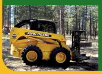
Butler likes the 280s, which have high power ratings and are capable of handling the company's robust accessories. The company owns a high-flow machine to run these attachments, which include a timber ax, a rotary chipper for chipping residue on the forest floor, and a hot saw, which is a rotating carbide-tip disk for cutting trees at ground level. The company also uses brush rakes and log forks.
