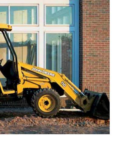
Another Sumner customer, Dekco, uses its 110 to install septic tanks, mostly for residential systems and some commercial systems. Dekco also owns two 35C ZTS Compact Excavators. With the quick-coupler system, the 110 has full bucket compatibility with the compact excavators. The three machines work in tandem, with the compact excavator digging trenches and the 110 backfilling.
